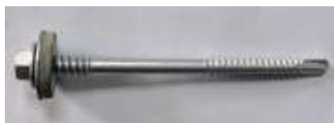
Light Section No. 2 point self drilling screw for drilling cold rolled steel sections 1.2 to 3.6mm thick.also includes fixing Brick Tie channel & insulation to metal framing systems.
