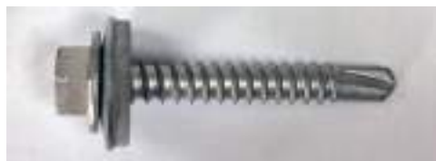
Light Section No. 2 point self drilling screw for drilling cold rolled steel sections 1.2 to 3.6mm thick.
