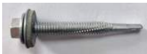
Heavy Section No. 5 point self drilling screw for drilling hot rolled steel sections 6.0 to 12.5mm thick.
